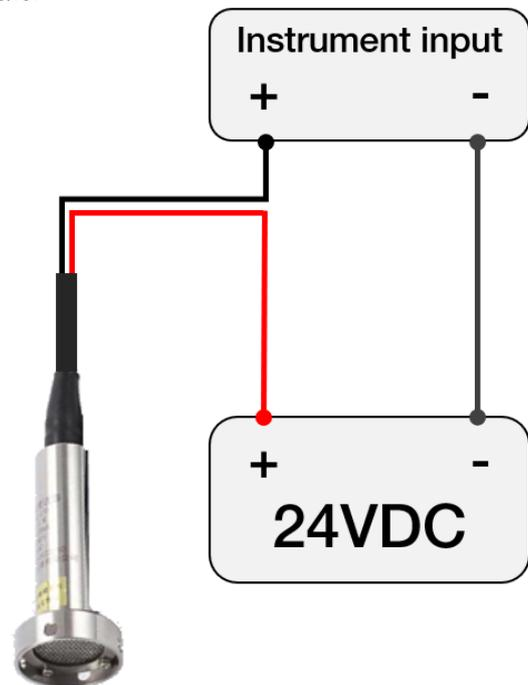
This level sensor outputs a relative water level value. The instrument makes no compensation for changes in atmospheric pressure.
